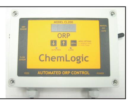
The CL200 WTC is housed in a NEMA 4x watertight enclosure with water tight connectors provided for the following inputs and outputs: 6'3 prong power input cord, contact closure, and standard BNC sensor input.
